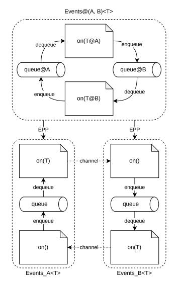
**Figure 10** Architecture of the full-duplex asynchronous choreographic pattern. Events are stored within two queues whose events are processed by two concurrently-running event handlers, represented by the choreographic methods on(T@A) and on(T@B). Notice how each role gets the projections of each event handler, a consequence of the behaviour of both roles being involved in both of the handlers.
